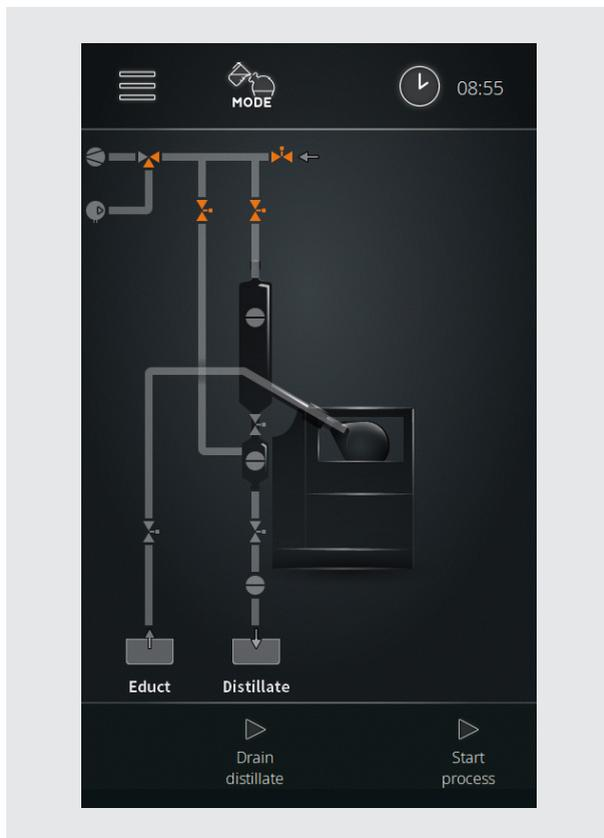
In manual mode, single batches can be processed. For automatic filling of the evaporation flask and draining of the distillate, the **Drain distillate** and **Start process** buttons are available on the operating panel.
